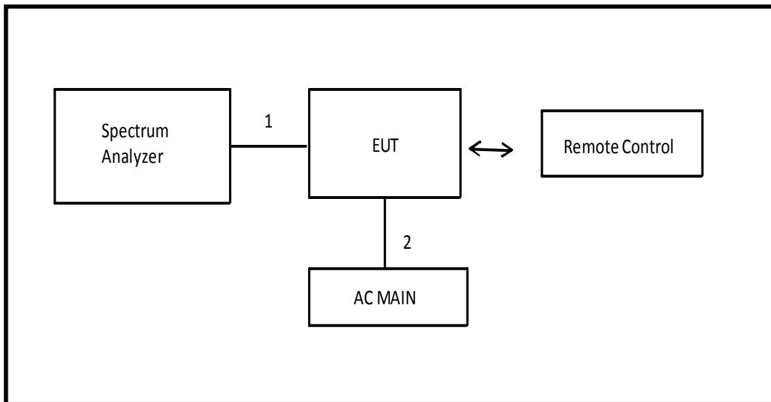
**SETUP DIAGRAM FOR RADIATED TEST**
