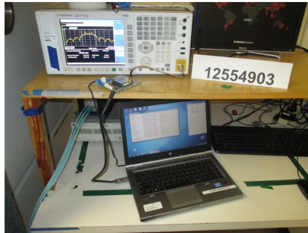
RF ANTENNA PORT CONDUCTED
