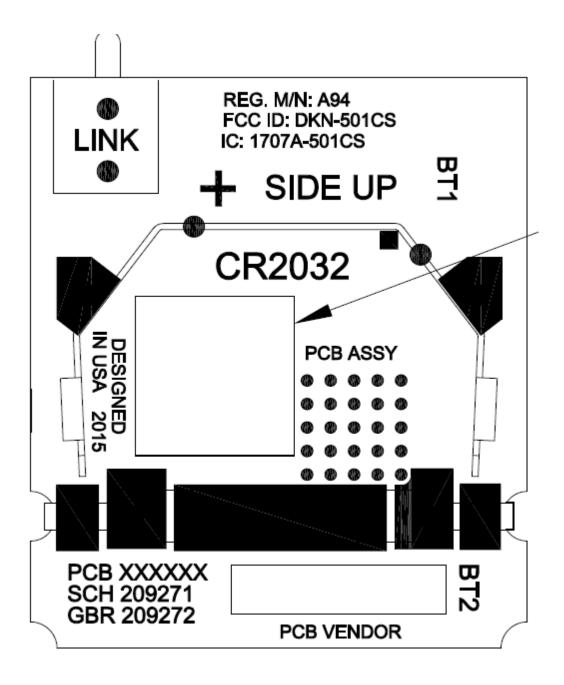
FCC/IC IDs are located in silkscreen on the PCB in the battery compartment and are accessible to the user when the unit cover is removed. Cover removal by the user is required to change battery. Cover removal does not require a special tool.
