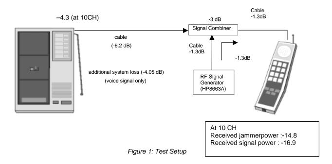
For DBPSK at 10<sup>-3</sup> bit error rate the required SNR is 8.0 dB. Using the results above and the data in the table below the processing gain is calculated to be 12.1 dB.
