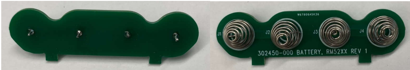
Battery Contact PCA for RM520C, RM540C, RM520S, and RM540S
