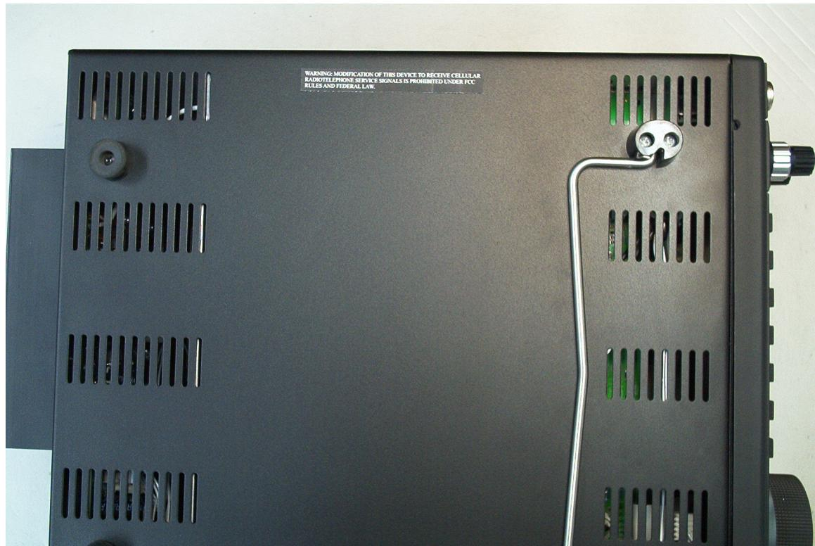
This view of the Model 588 shows the location of the warning label as required by FCC Part 15 Doc Section 15.121 (f). The label reads as follows and the sample is provided in the label sample file.
