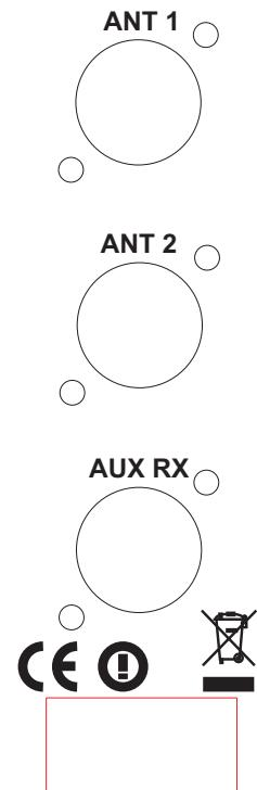
This document provides a view of the rear panel of the radio. This drawing is black on white. The actual rear panel will be painted black with white lettering. The FCC ID and compliance statement will be on a label with a permanent adhesive. The label will be black with white lettering. The location is shown above. See the label sample file for the actual look and size of label.
