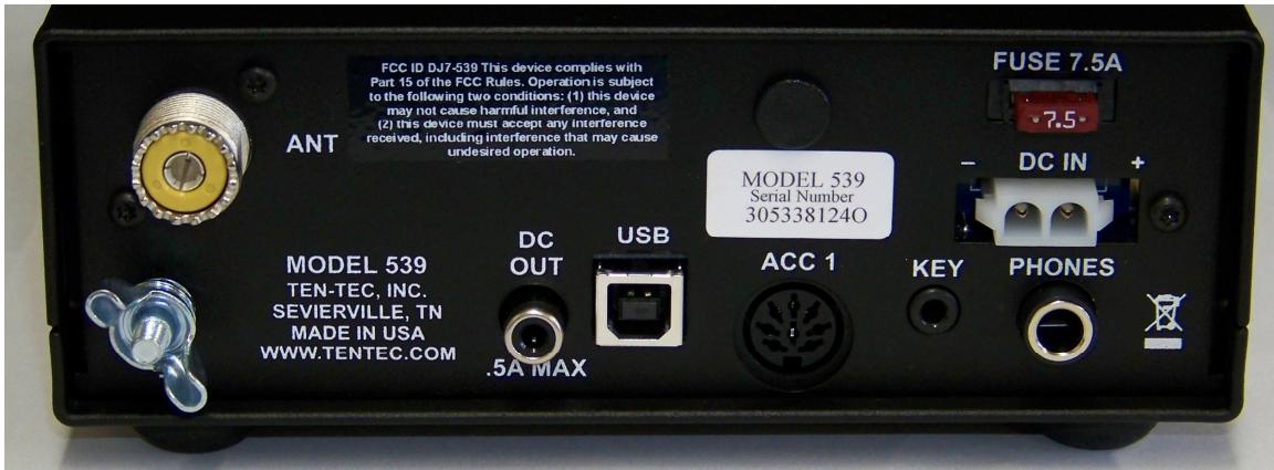
This view of the Model 539 Rear Panel shows the location of the FCC ID label with compliance statement as required by Section 15.19 (a) (3). A sample of the label is provided in the label sample file.
