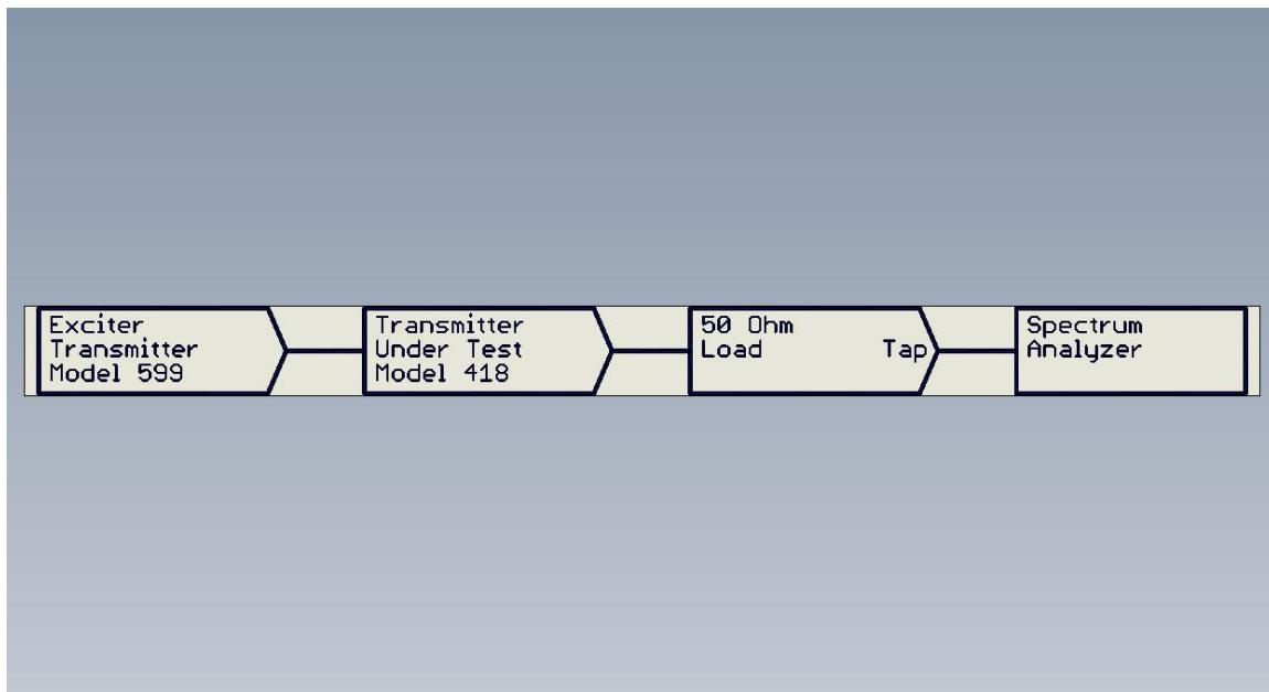
The setup to measure the strength of spurious emissions was made by connecting the output of a Ten-Tec Model 599 transceiver (the exciter) to the input of the Ten-Tec Model 418 amplifier. A 50 ohm load was connected to the amplifier, and a spectrum analyzer was connected to the 50 ohm load. The exciter was tuned to the frequency shown and each harmonic of that frequency up to the tenth was observed on the spectrum analyzer.
