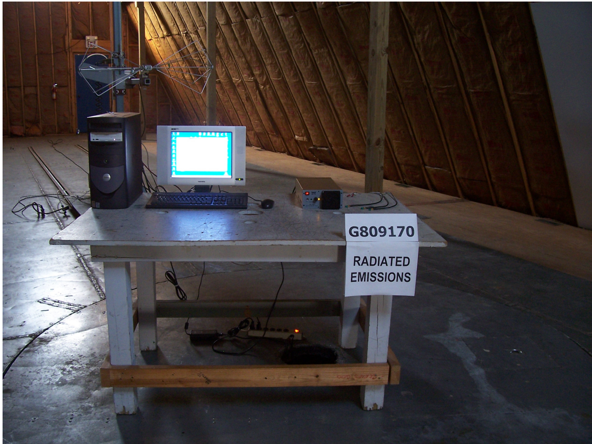
EUT and support equipment in the test site with the antenna used to measure the radiated emissions from 30MHz to 250MHz as recommended by ANSI C63.4 2003
