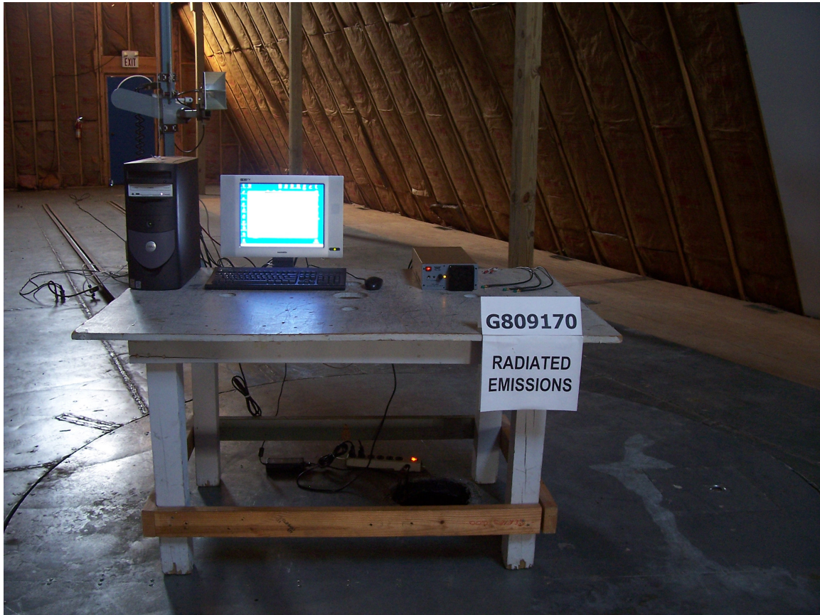
EUT and support equipment in the test site with the antenna used to measure the radiated emissions from 1GHz to 18GHz as recommended by ANSI C63.4 2003
