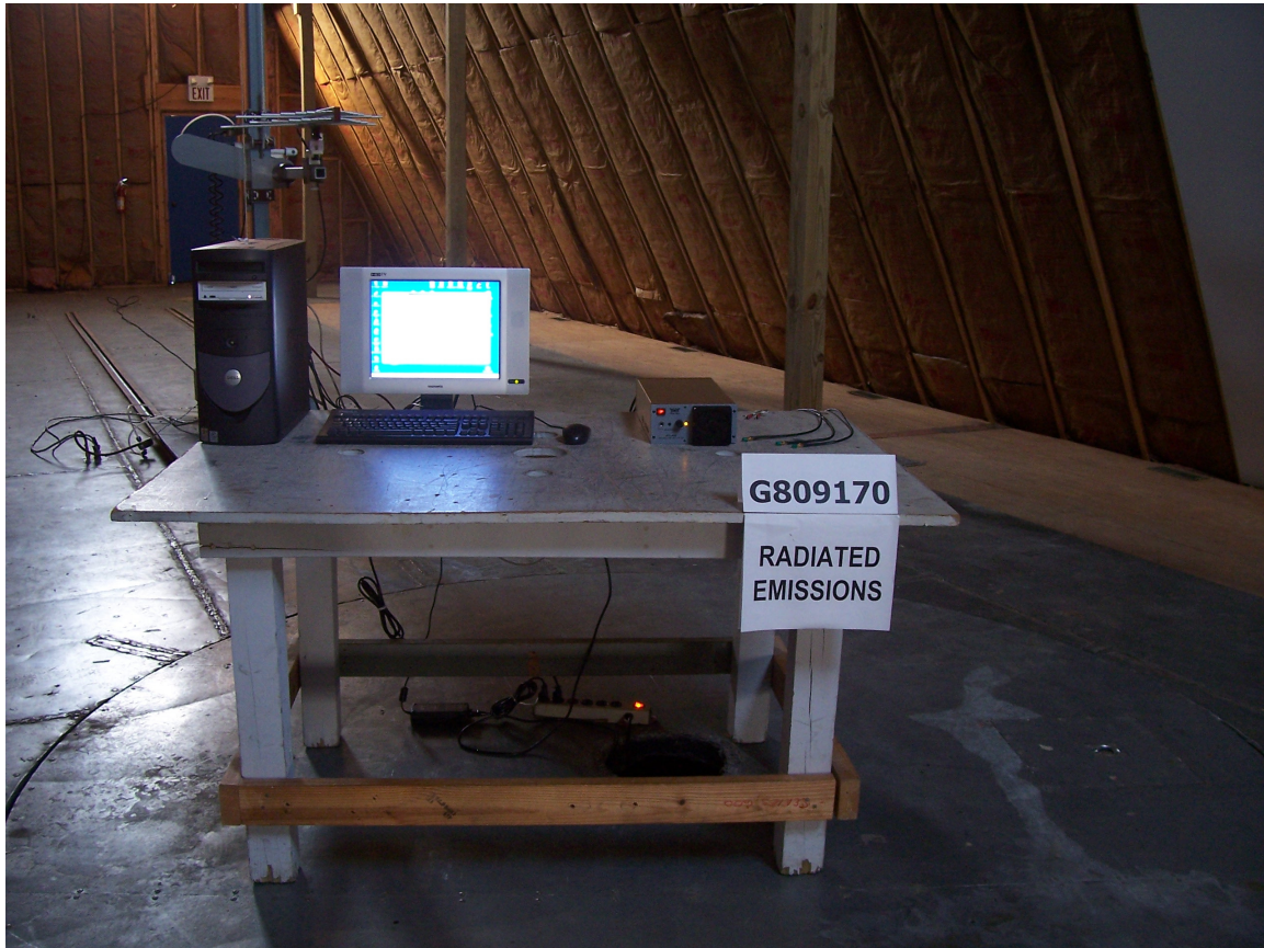
EUT and support equipment in the test site with the antenna used to measure the radiated emissions from 250MHz to 1GHz as recommended by ANSI C63.4 2003
