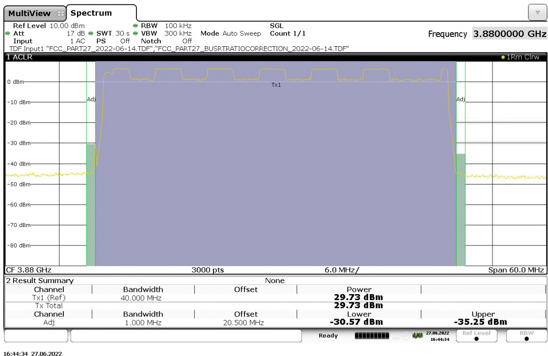
Figure 227: Out-of-Band Emission, 1cc-1 (OBW=40MHz), High Channel, 16QAM_TM3.2, TX Port 24
