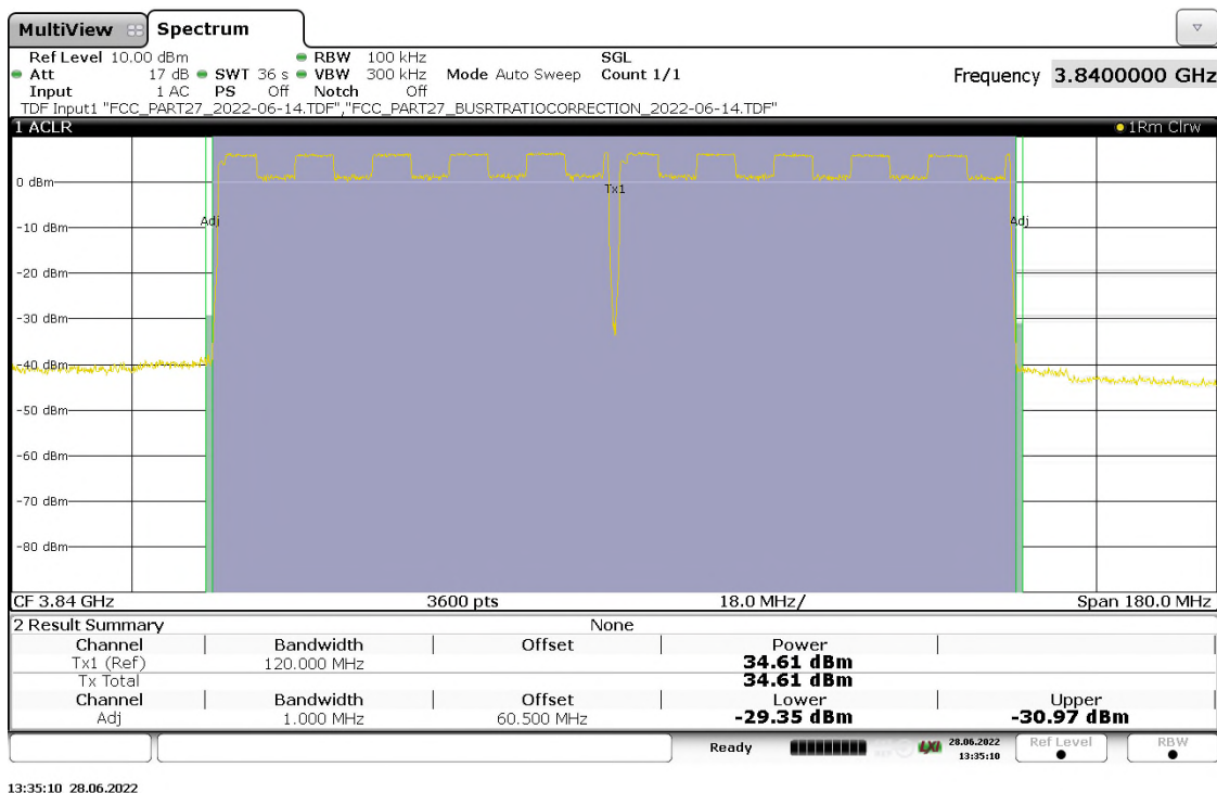
Figure 237: Out-of-Band Emission, 2cc-2b (OBW=60MHz+60MHz), High Channel, 16QAM_TM3.2, TX Port 24
