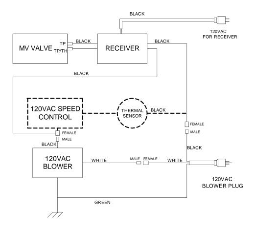
Connect the two 30" long 18AWG wires labled "110VAC FAN ONLY" between receiver and blower as shown in the follwing diagram as well.
