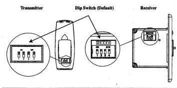
Do not use two (2) or more remote control systems in the same area with the same dip switch settings, as they will communicate with each other. This may cause the appliances to malfunction.
