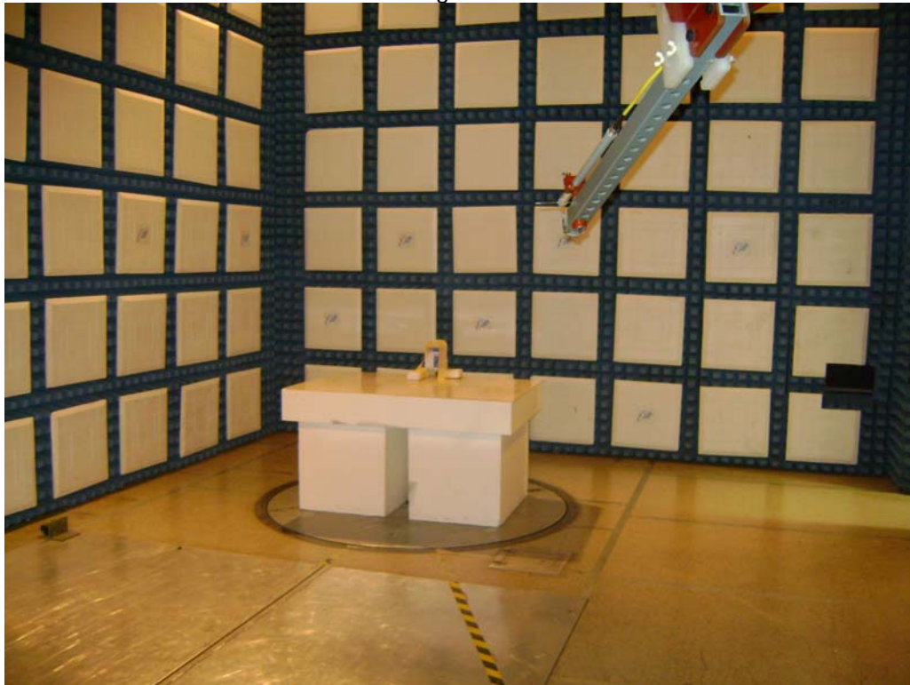
Test Setup for Radiated Emissions – 908MHz - Horizontal Polarization - Transmitter
