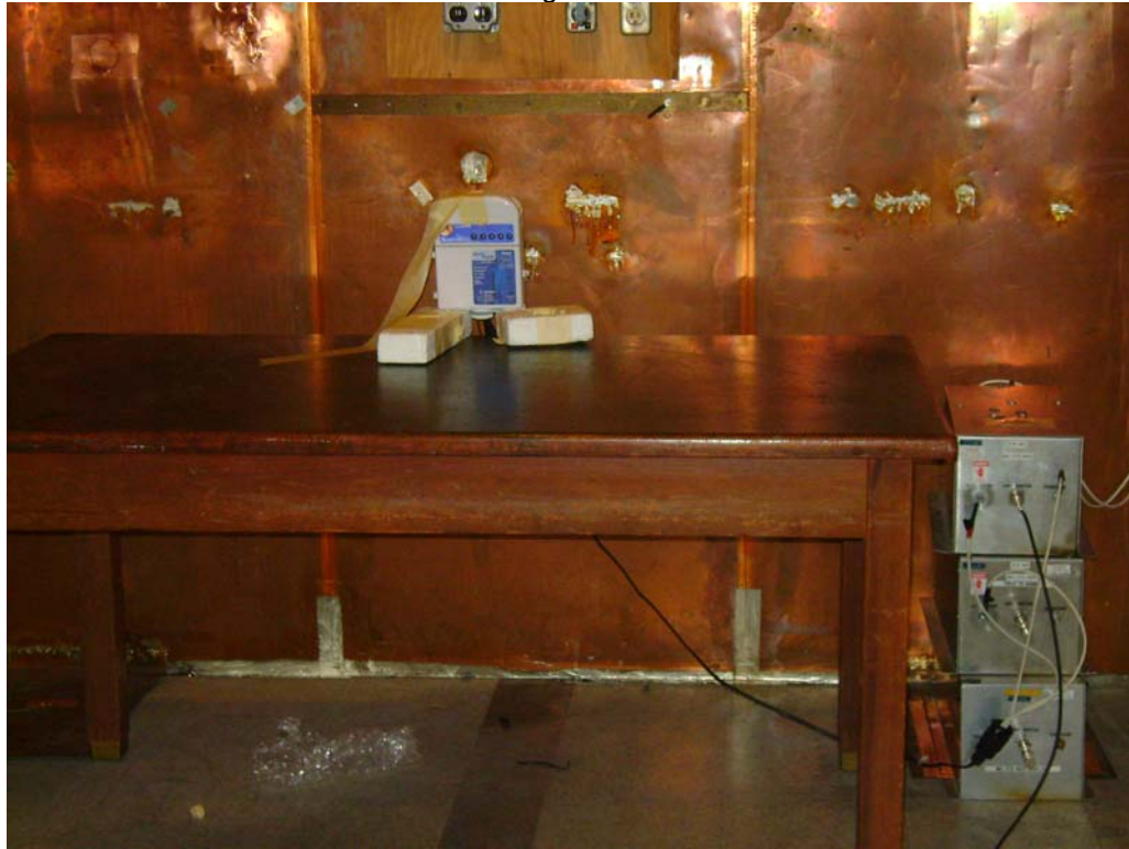
Test Setup for Conducted Emissions
