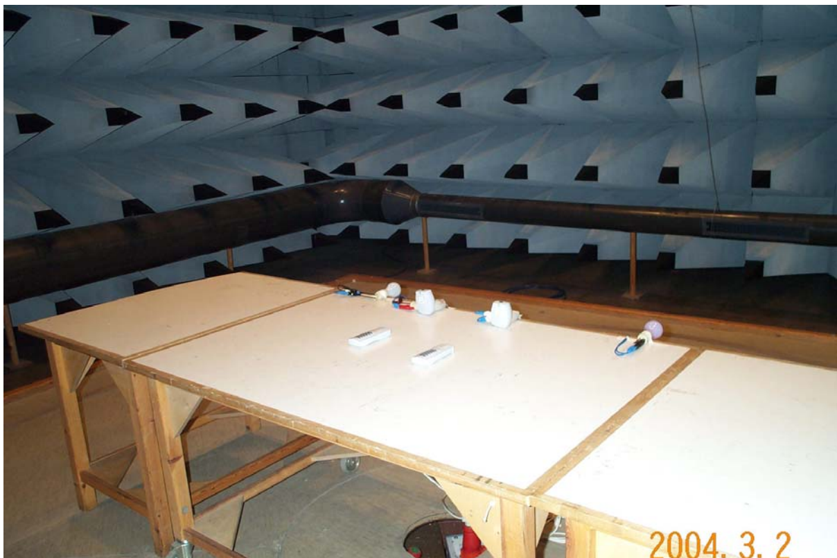
Photo 4 Test set-up for measurement of HA09 receiver. A similar product, HA03, is lined up in the background.
