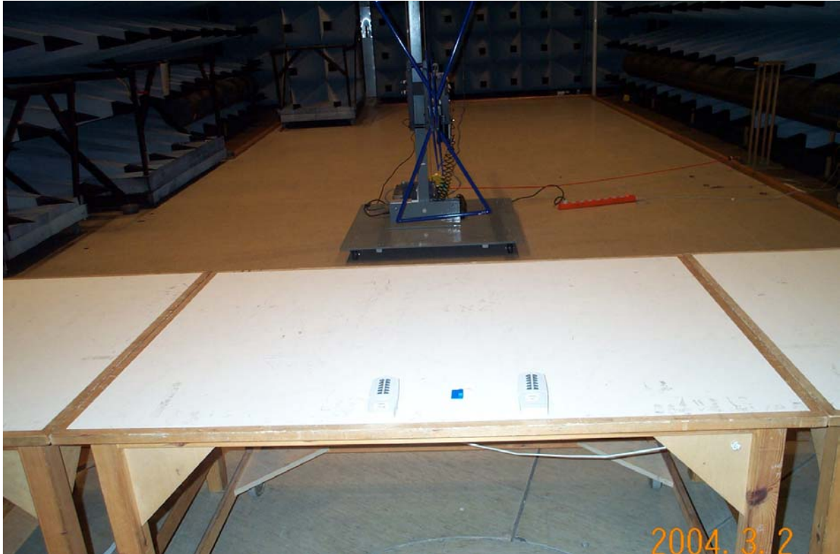
Photo 1 Set-up for measurements 30 - 1000 MHz. Date is correctly 2004-02-13.
