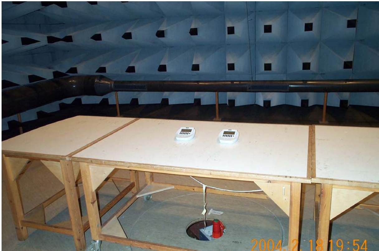
Photo 1 Set-up for emission measurements. Constant TX CW unit and constant Rx unit.
