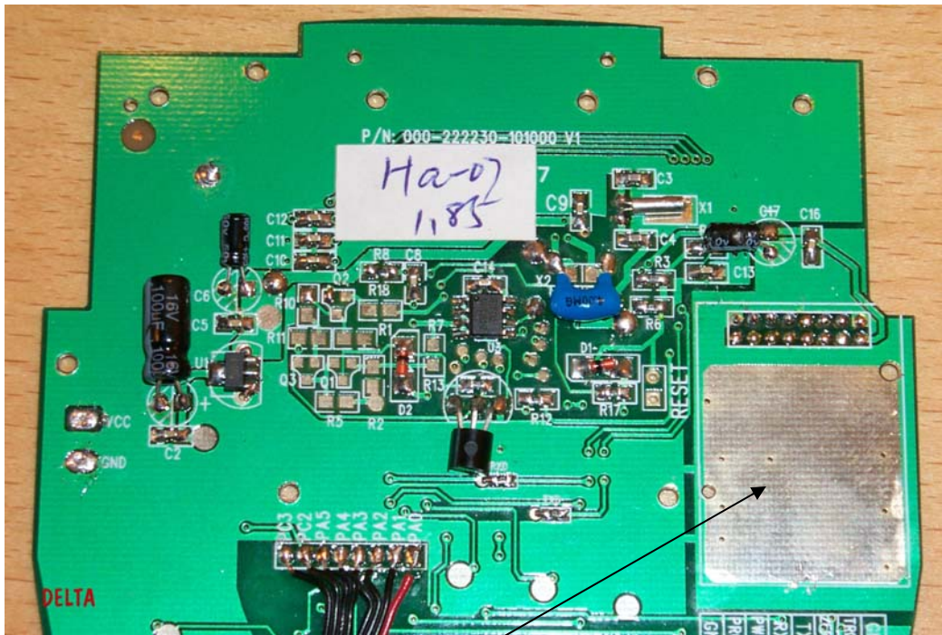
Photo 2 Main board. RF module removed.
