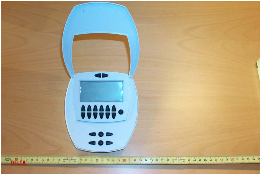
Photo 3 HA07 front view with lower set of push buttons uncovered
