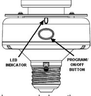
4. To manually turn OFF the **HA05 Screw-in Lamp Module**, simply press and release the Program/ON/OFF button. The green indicator will turn OFF and the lightbulb screwed into the **HA05 Screw-in Lamp Module** will also turn OFF.
