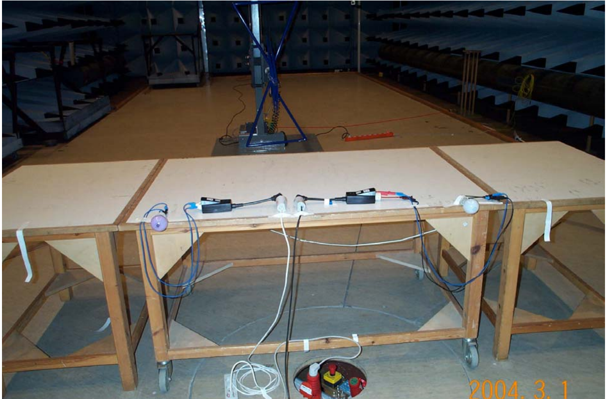
Photo 3 Set-up for measurements 30 – 1000 MHz. Date is 2004-02-12 Camera wrongly set.
