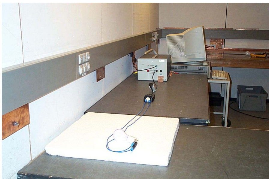
Photo 2 Set-up for conducted emission. Measurements performed in screened room. LISN bonded to vertical ground plane (wall).
