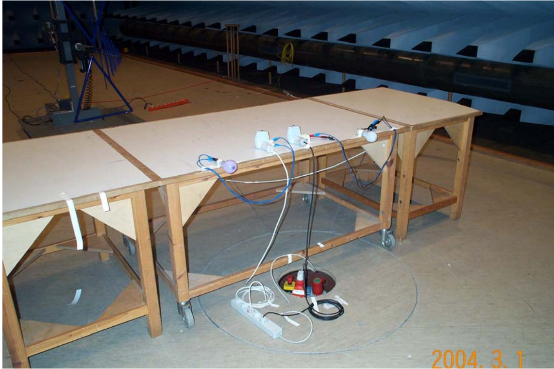
Photo 3 Set-up for measurements 30 – 1000 MHz. Date is 2004-02-12. Camera time is faulty.
