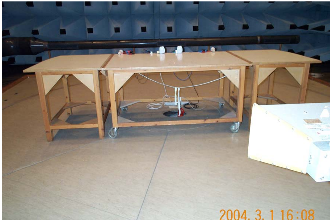
Photo 4 Measurement set-up > 1 GHz.
