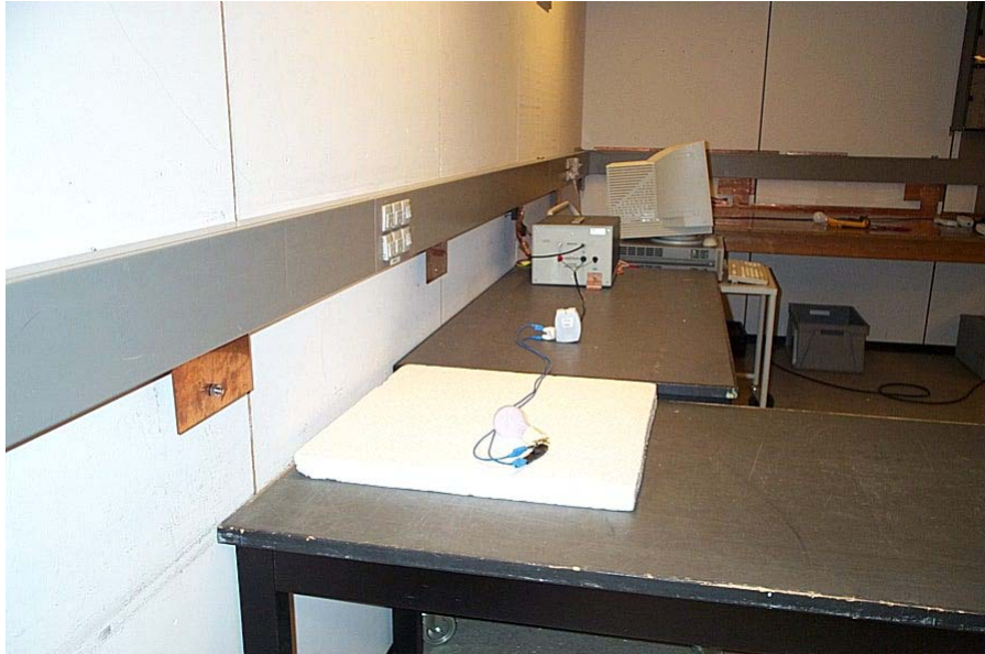
Photo 1 Set-up for conducted emission measurements. The LISN is bonded to the vertical ground plane (wall) of the screened room.
