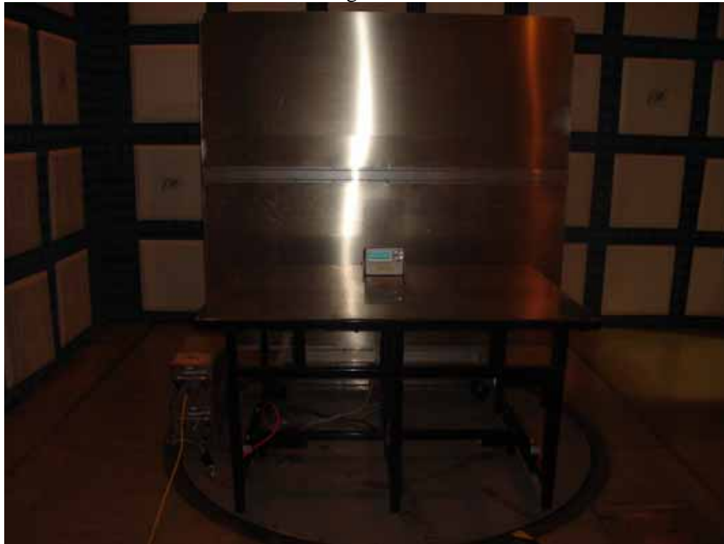
Test Setup for Conducted Emissions
