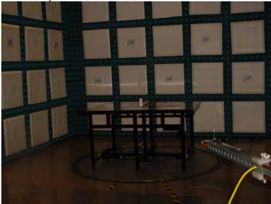
Test Setup for Radiated Emissions, 908MHz – Vertical Polarization
