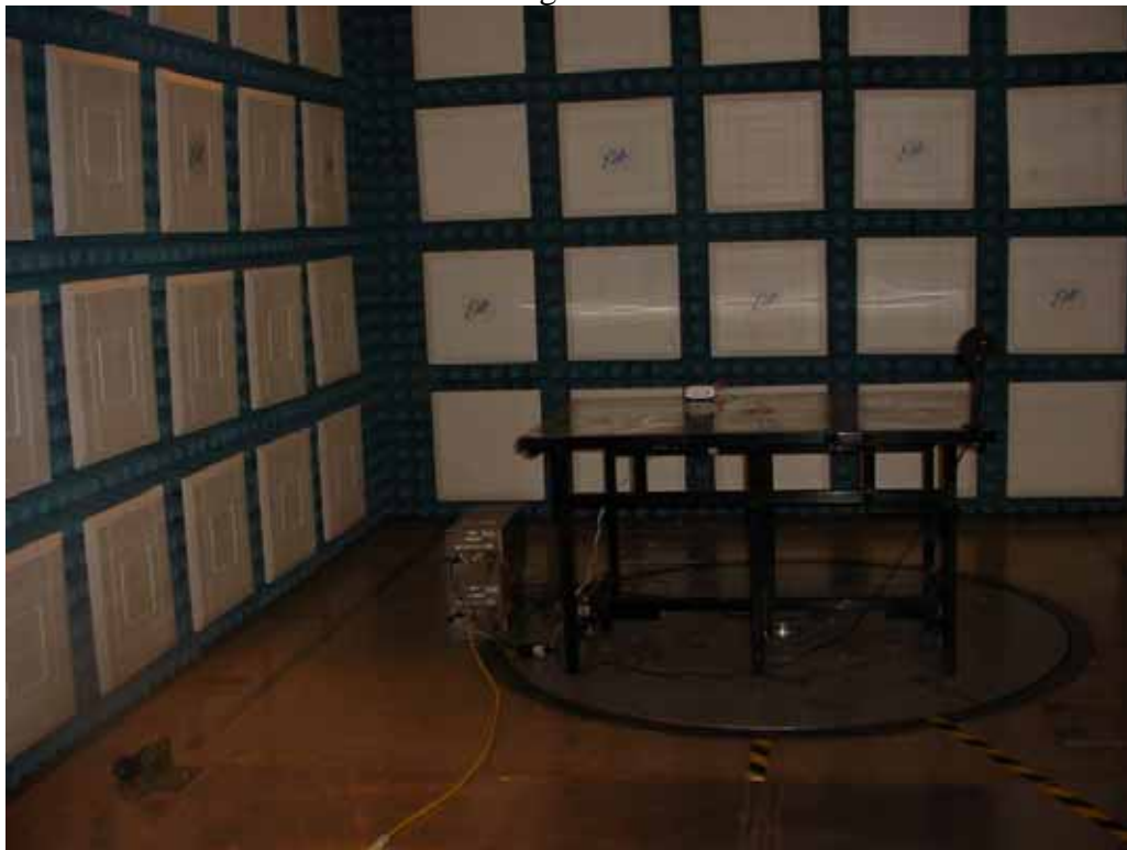
Test Setup for Conducted Emissions
