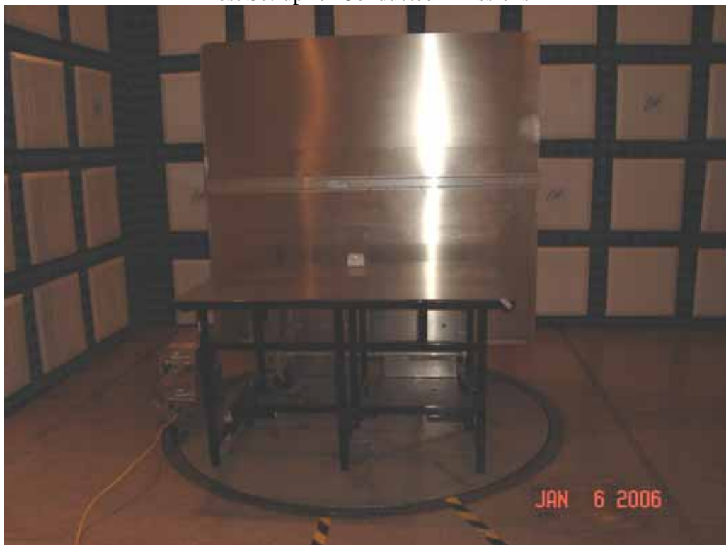
Test Set-up for Conducted Emissions
