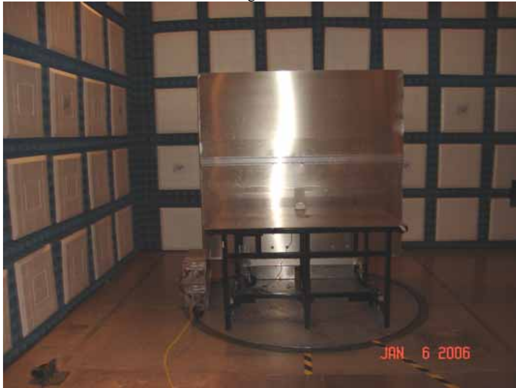
Test Set-up for Conducted Emissions
