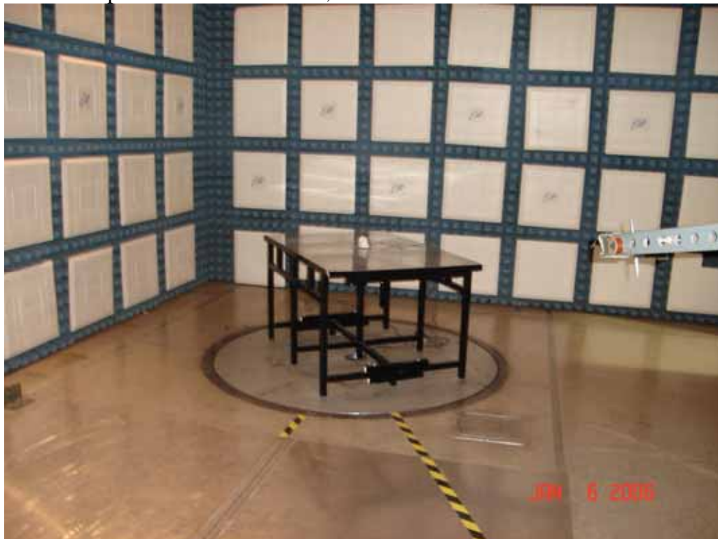
Test Set-up for Radiated Emissions, 30MHz to 1GHz – Vertical Polarization
