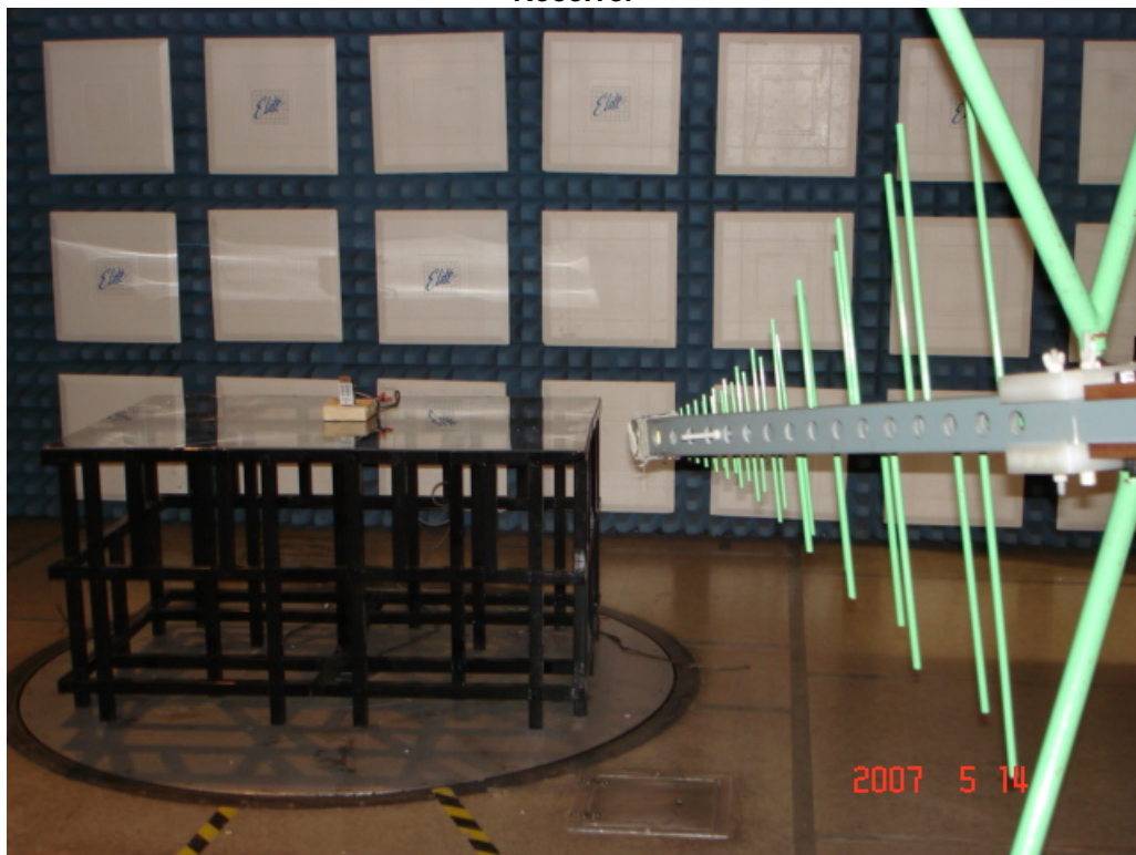
Test Set-up for Radiated Emissions – 30MHz to 1GHz - Vertical Polarization - Receiver
