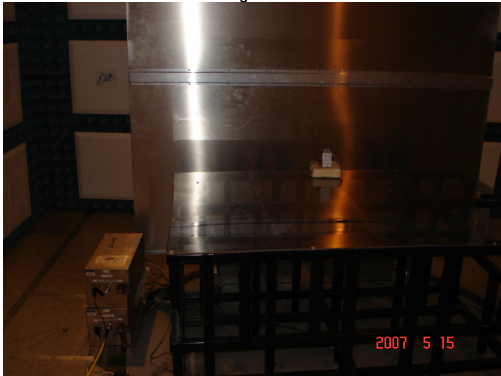
Test Set-up for Conducted Emissions
