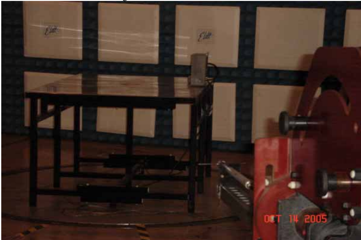
Test Set-up for Radiated Emissions, 908.3MHz – Horizontal Polarization
