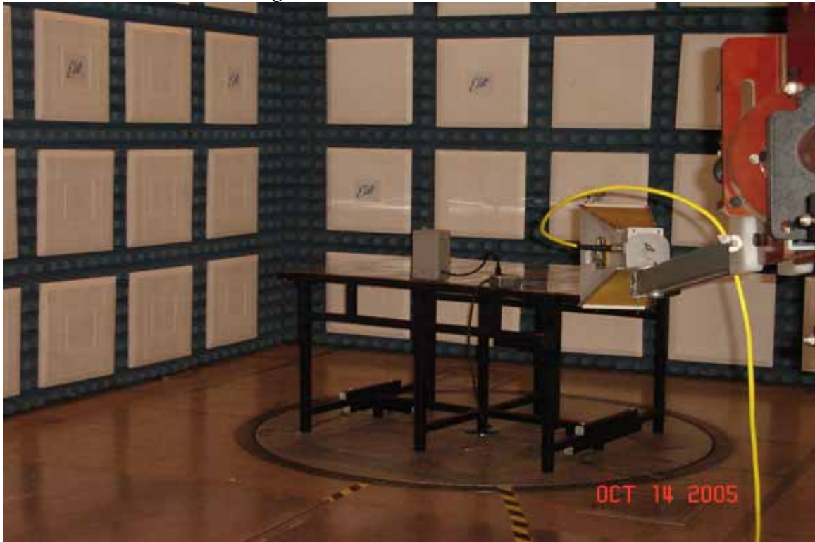
Test Set-up for Radiated Emissions, 1GHz to 9.1GHz – Horizontal Polarization
