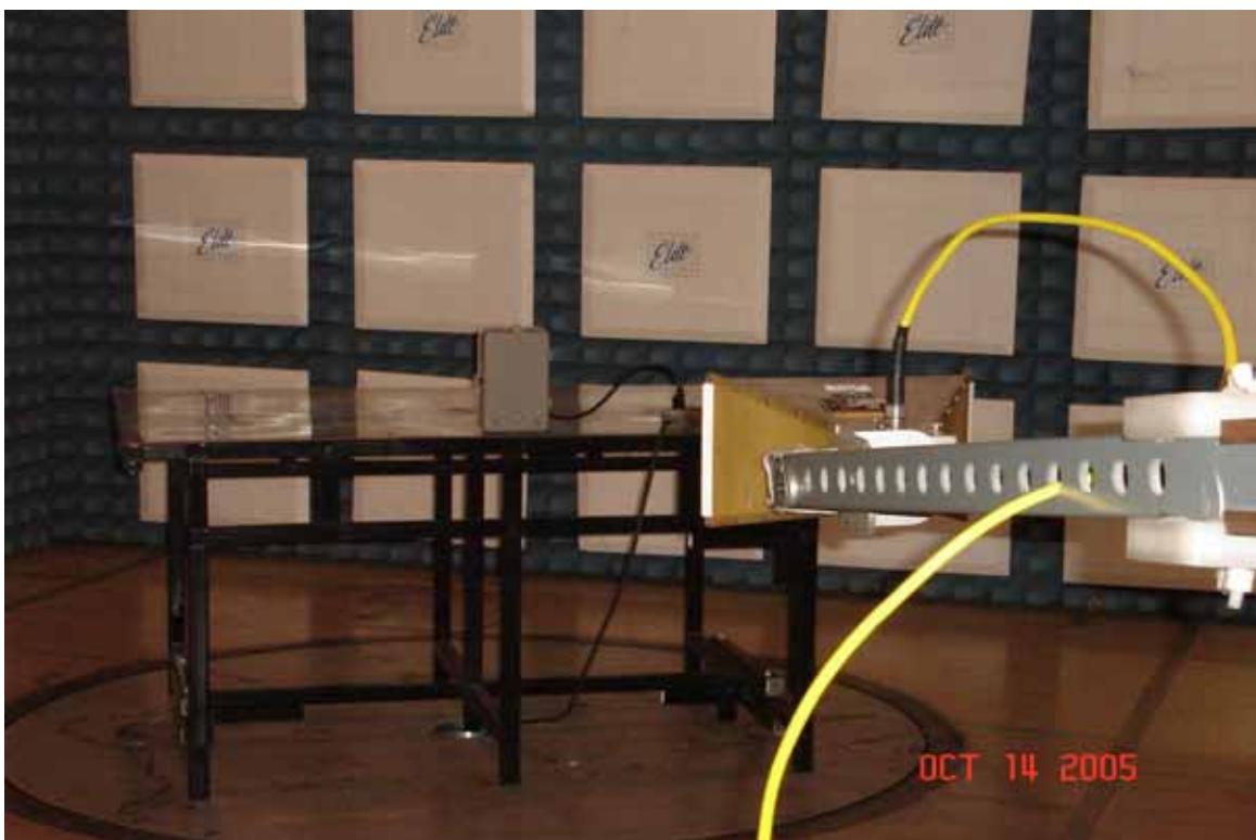
Test Set-up for Radiated Emissions, 1GHz to 9.1GHz – Vertical Polarization
