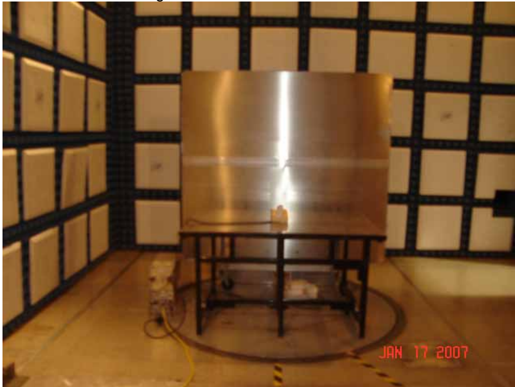
Test Set-up for Conducted Emissions
