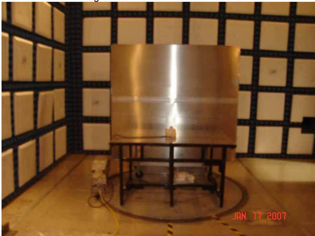
Test Set-up for Conducted Emissions
