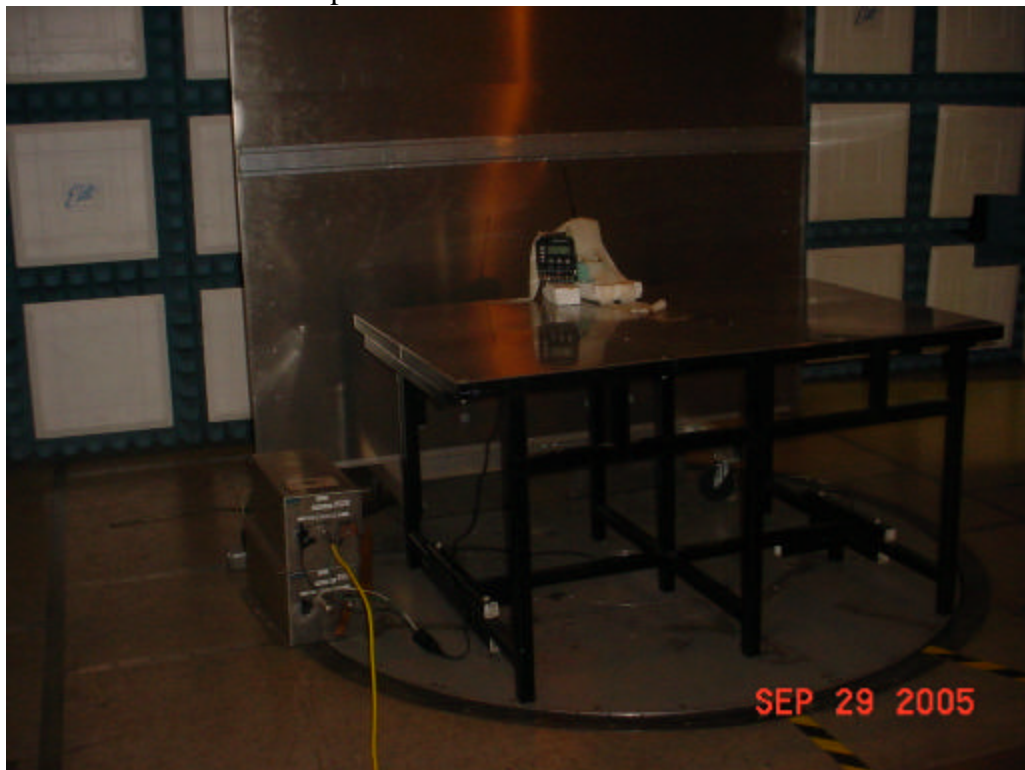
Test Setup for Conducted Emissions – P1353ME
