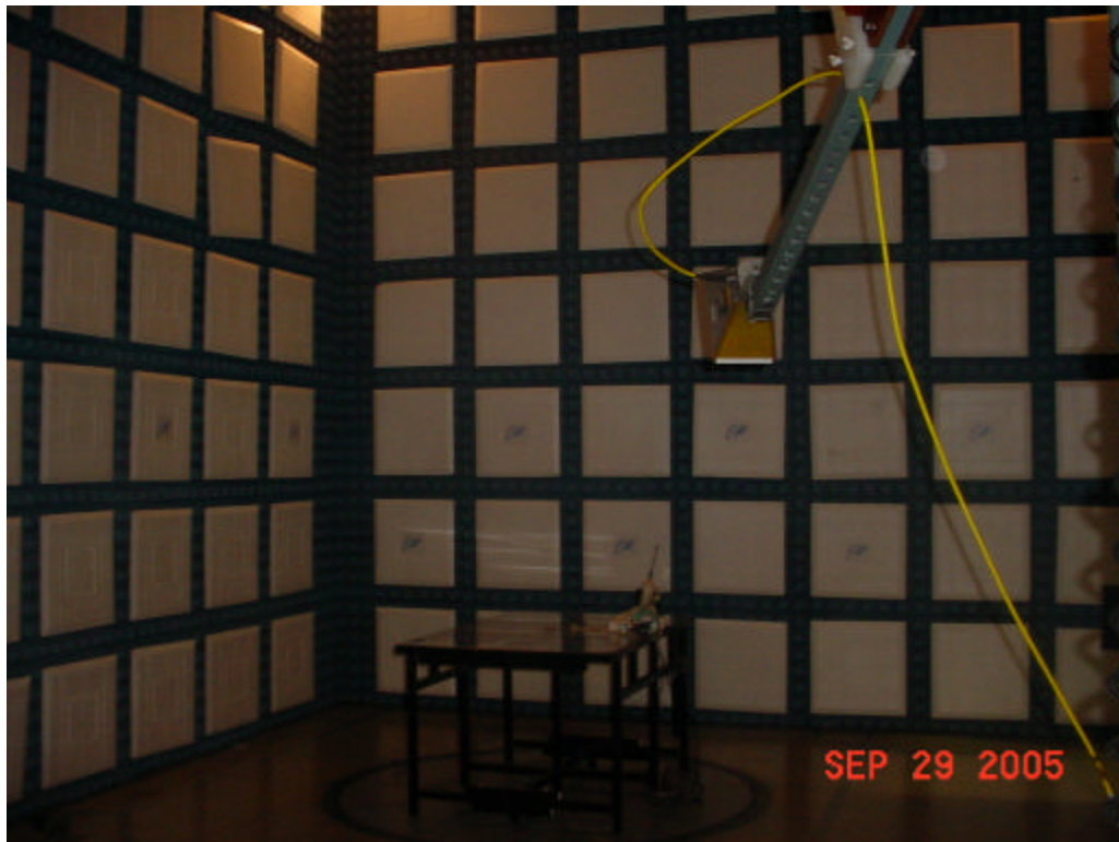
Test Setup for Radiated Emissions, 1GHz to 9.1GHz – Horizontal Polarization
