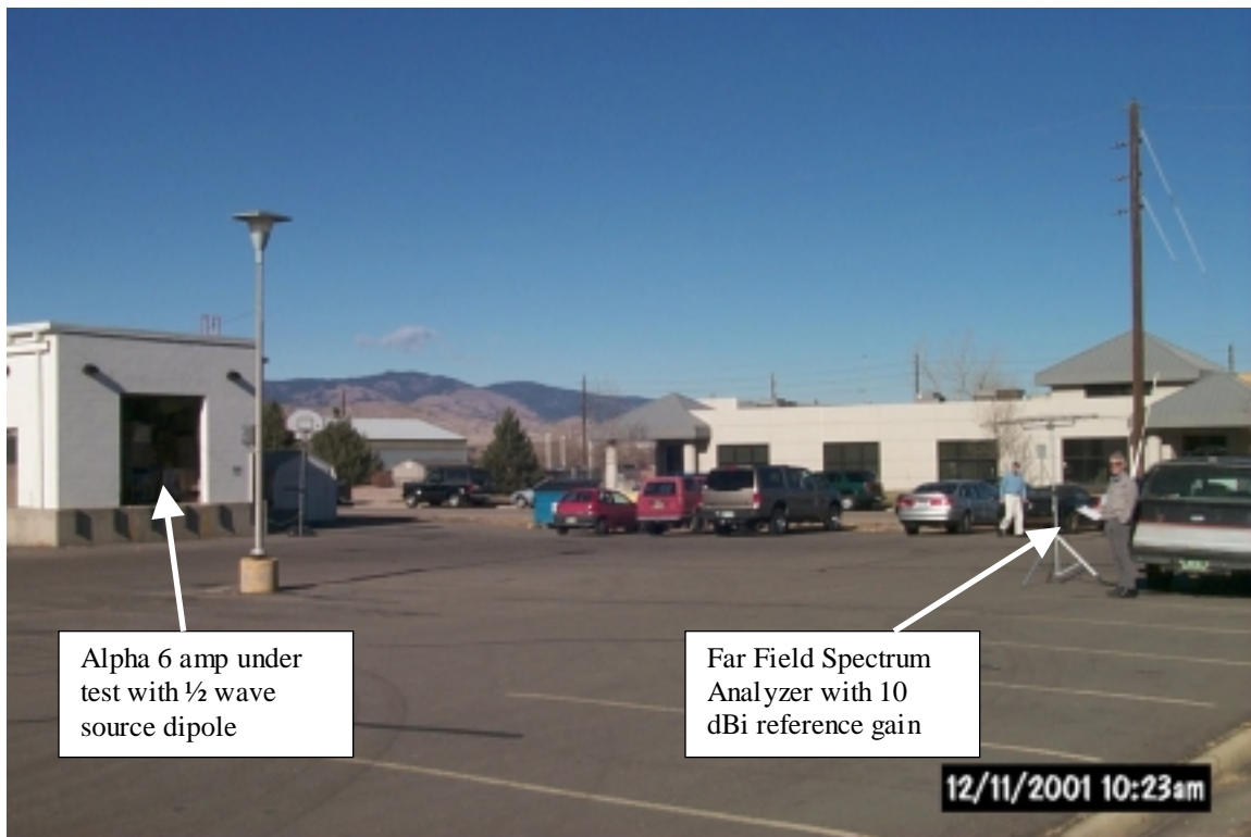
Figure 3.4.1-1 Far field test set-up
