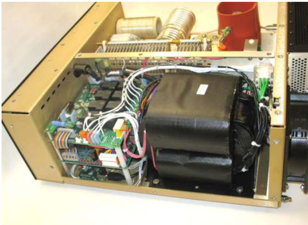
Power Supply Side of the Amplifier With Transformer Right Side.
