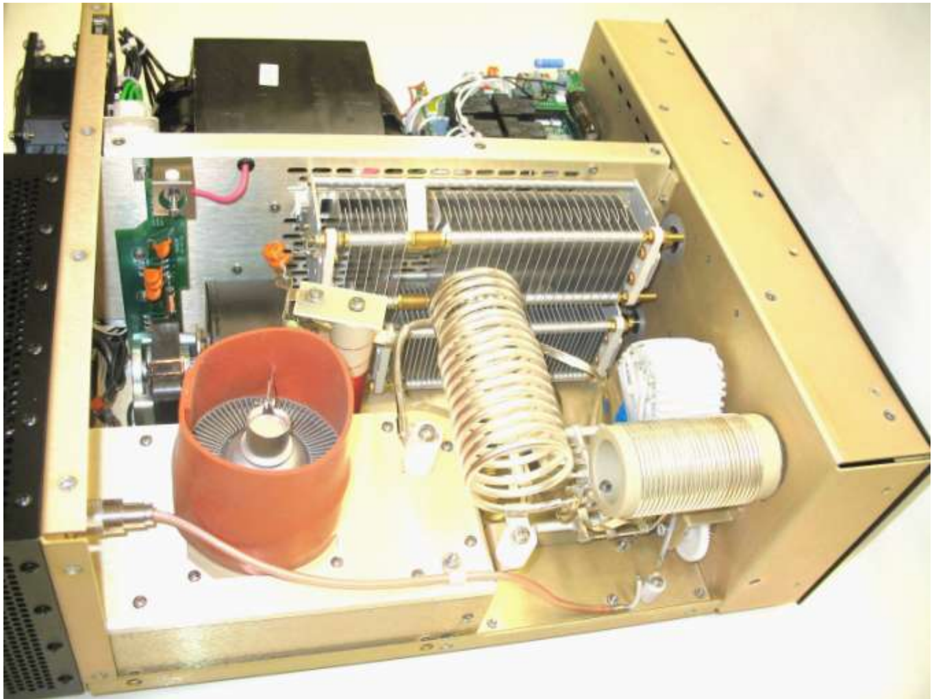
RF Tank and Tube Side of the Amplifier Left Side
