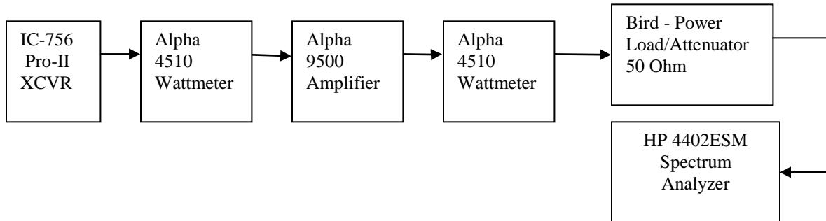
The drive source for this test is a currently available Amateur Radio transceiver manufactured by Icom, the Model IC-756 Pro II. It has adjustable output power up to about 100 watts across the 1.8-29.7 MHz band. For RF power measurement, the Alpha 4510 model directional wattmeter was chosen for both input and output power measurements. Typical Accuracy is +/- 4%
