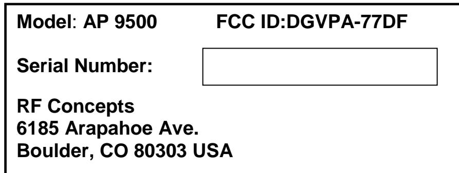
Note: The above drawing is not to scale. It is shown in expanded view for clarification purposes only. The FCC ID number will be located on the outside rear panel of the Amplifier. The Proposed FCC ID is **DGVPA77DF**. The FCC ID will be printed in black block lettering on the gold-anodized chassis finish in a font size of eight-point (or greater).
