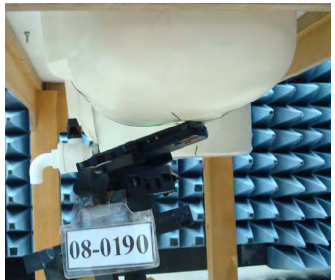
Figure 17. Left Head SAR Test Setup (Tilted)
