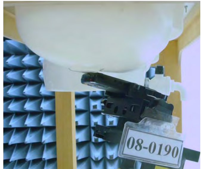
Figure 15. Right Head SAR Test Setup (Tilted)
