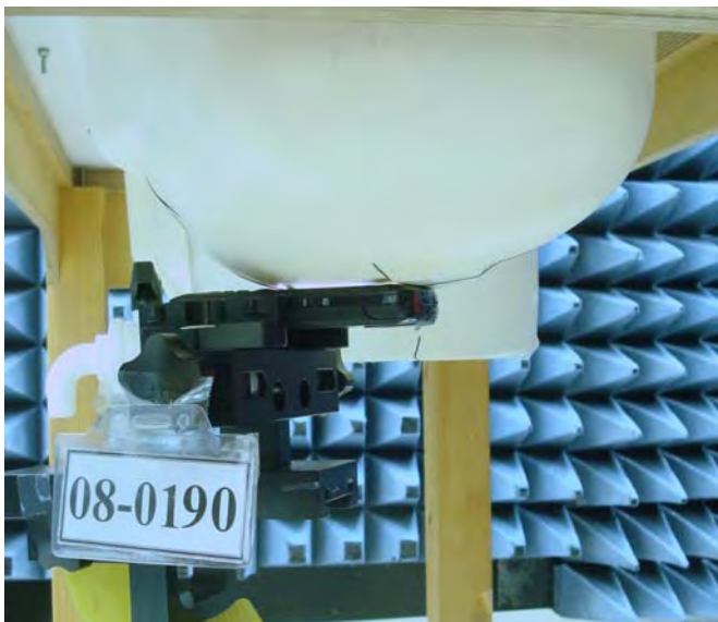
Figure 16. Left Head SAR Test Setup (Cheek)
