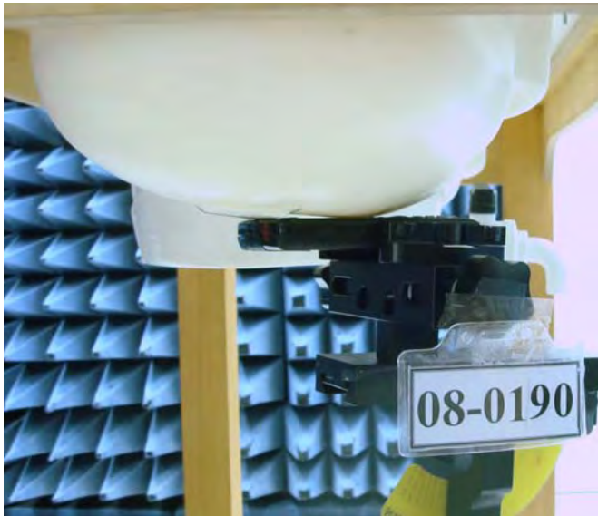
Figure 14. Right Head SAR Test Setup (Cheek)
