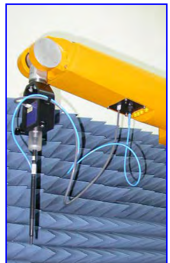
Figure 8. Probe setup on robot
