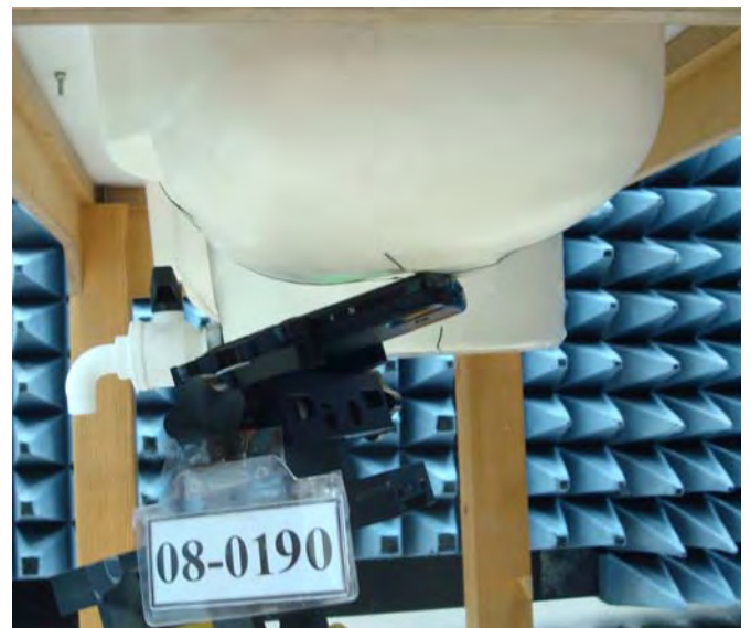
Figure 17. Left Head SAR Test Setup (Tilted)
