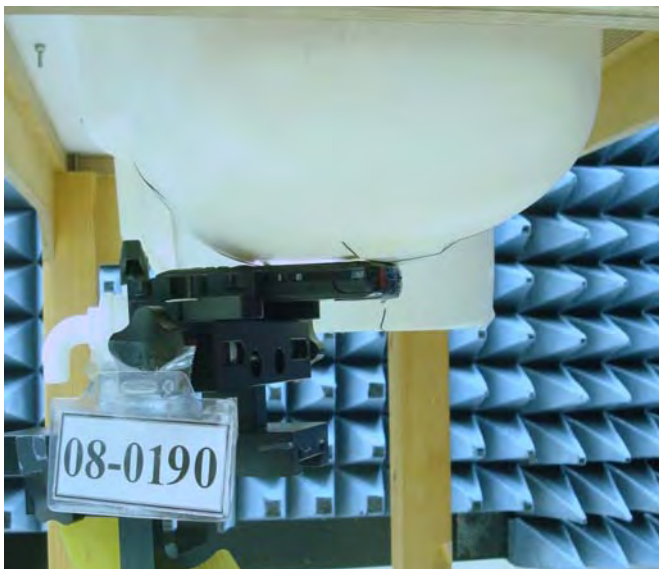
Figure 16. Left Head SAR Test Setup (Cheek)
