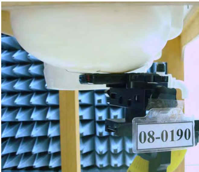
Figure 14. Right Head SAR Test Setup (Cheek)
