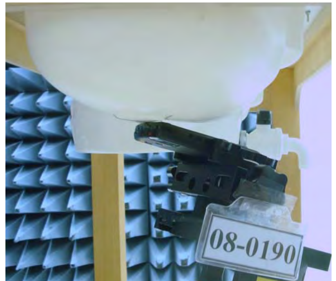
Figure 15. Right Head SAR Test Setup (Tilted)
