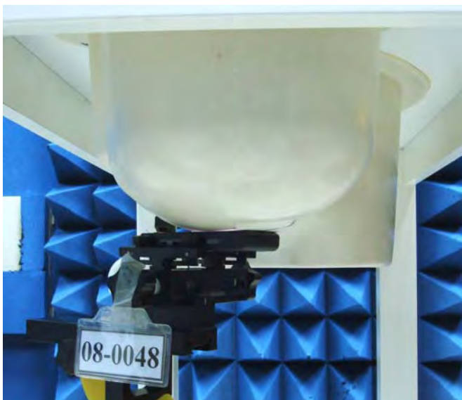
Figure 15. Left Head SAR Test Setup (Cheek)
