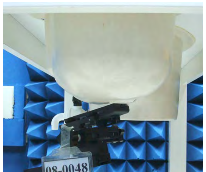
Figure 16. Left Head SAR Test Setup (Tilted)
