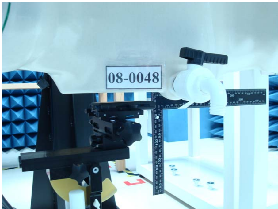
Figure 17.Body SAR Test Setup (Flat Section) _ 20 mm separation
