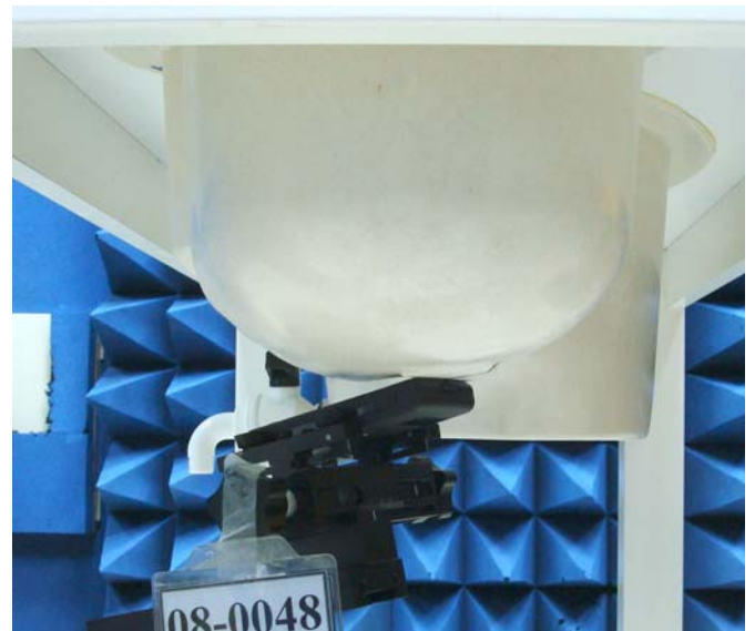
Figure 16. Left Head SAR Test Setup (Tilted)
