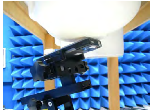
Figure 16. Left Head SAR Test Setup (Tilted)
