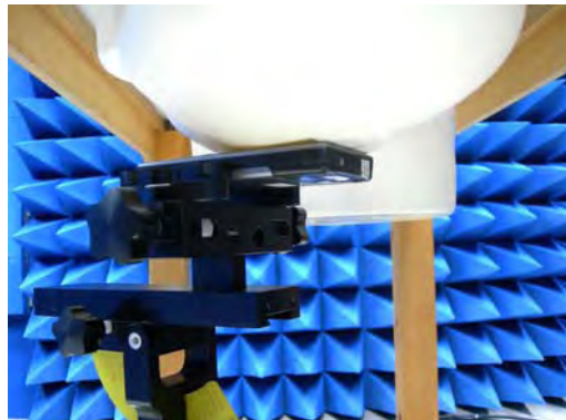
Figure 15. Left Head SAR Test Setup (Cheek)
