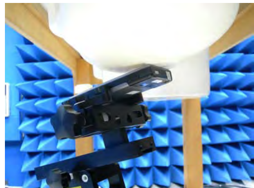
Figure 16. Left Head SAR Test Setup (Tilted)
