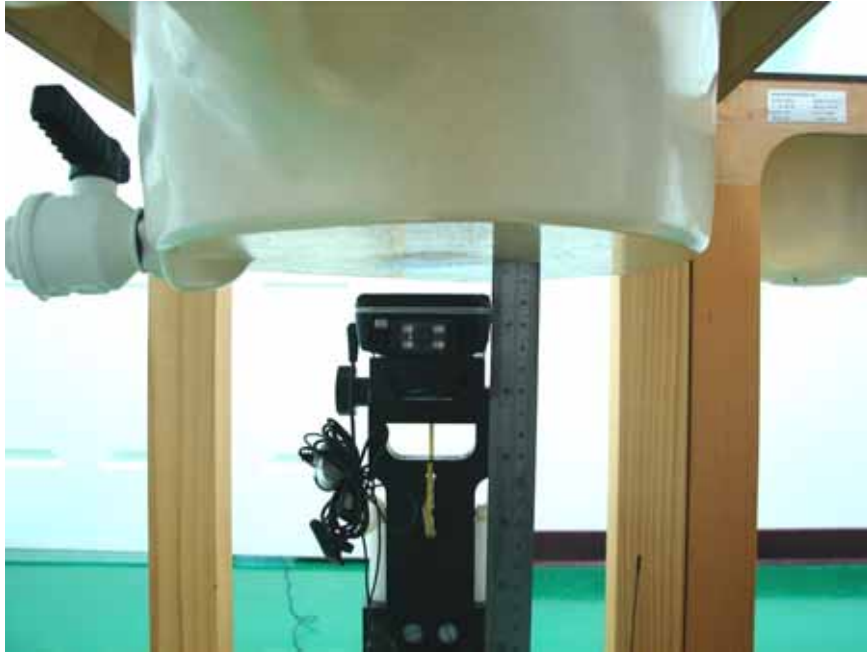
Fig. 9.7 Keypad Up with 1.5cm Gap for Scanner 1
