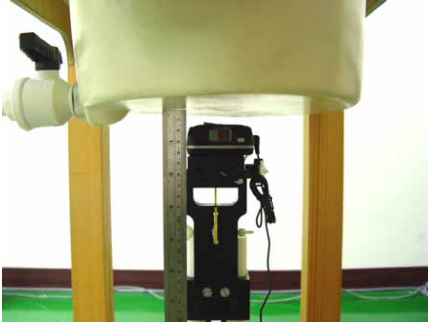
Fig. 9.9 Keypad Down with 1.5cm Gap for Scanner 2
