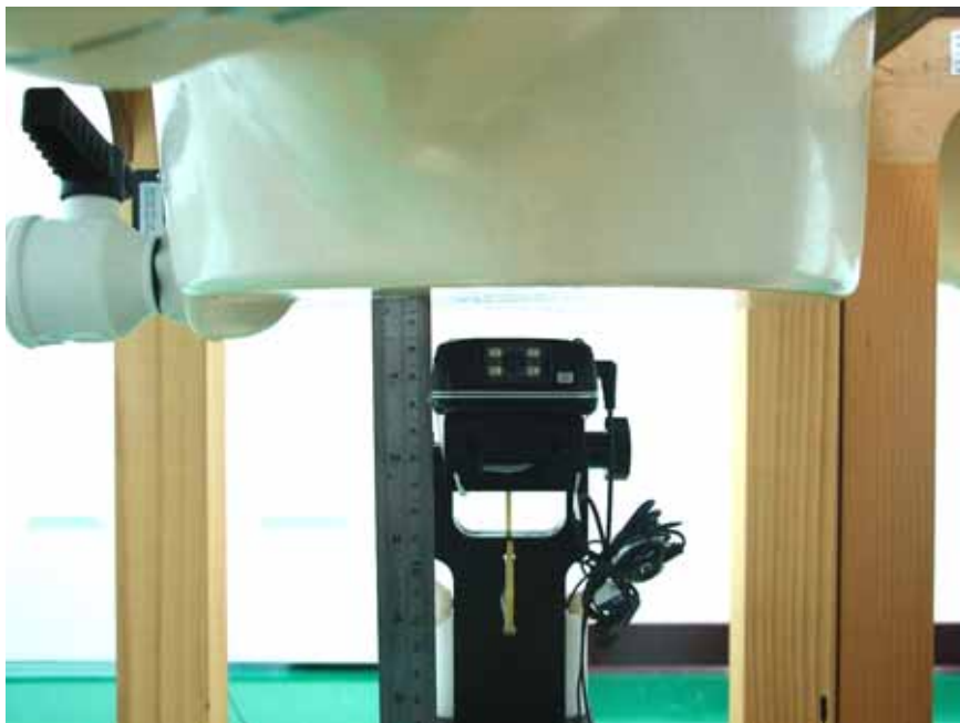
Fig. 9.8 Keypad Down with 1.5cm Gap for Scanner 1
