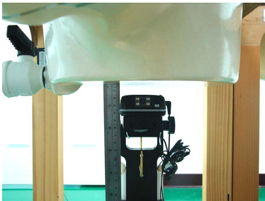
Fig. 9.8 Keypad Down with 1.5cm Gap for Scanner 1
