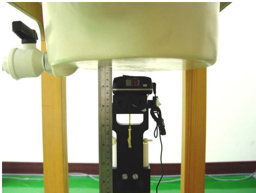
Fig. 9.9 Keypad Down with 1.5cm Gap for Scanner 2
