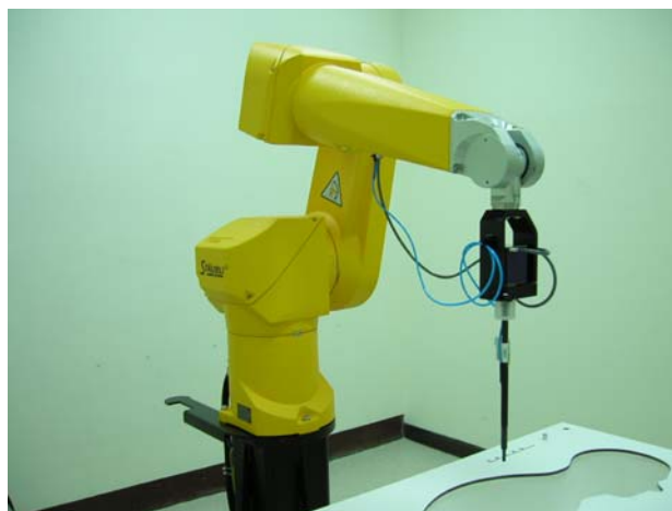
Fig. 5.2 Probe setup on robot
