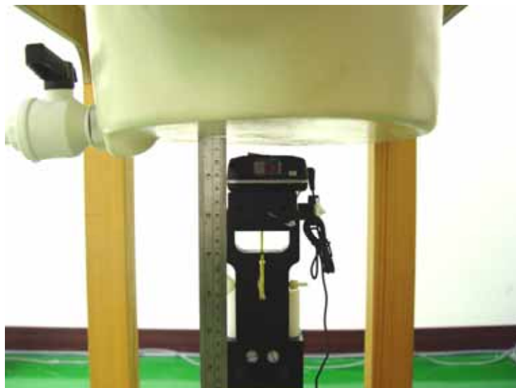
Fig. 9.3 Keypad Down with 1.5cm Gap for Scanner 2
