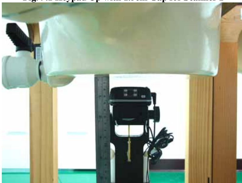
Fig. 9.2 Keypad Down with 1.5cm Gap for Scanner 1
