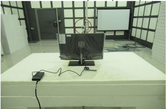
Radiated Emission Set up Photos (30MHz~1GHz)
