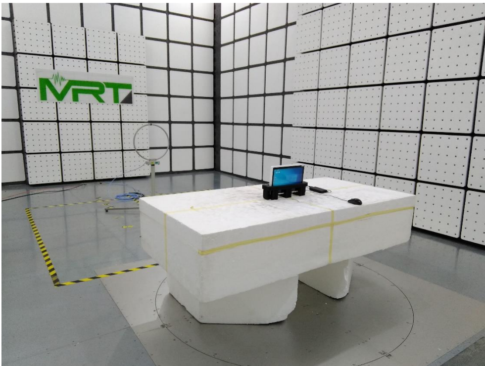
Description: Radiated Emission Test Setup for 9kHz~30MHz
