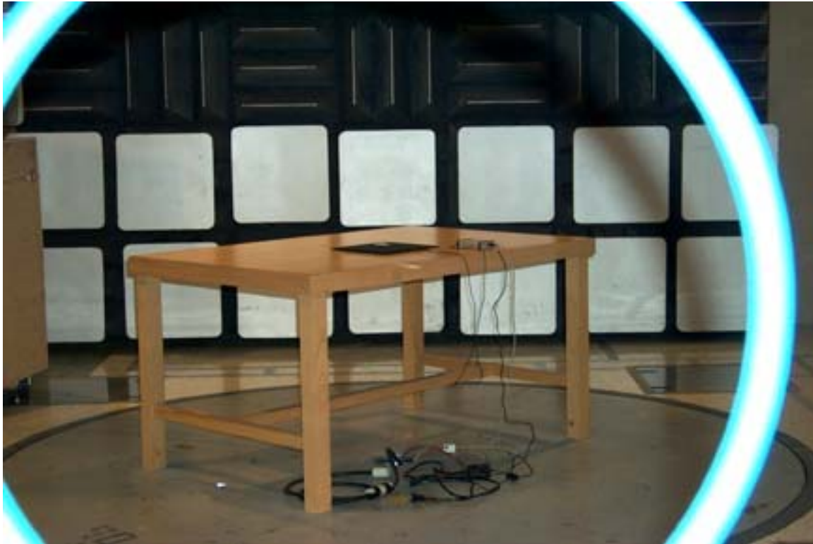
810 (P12 antenna) Carrier Frequency Emissions / Emissions Bandwidth / Spurious Emissions 9KHz to 30 MHz
