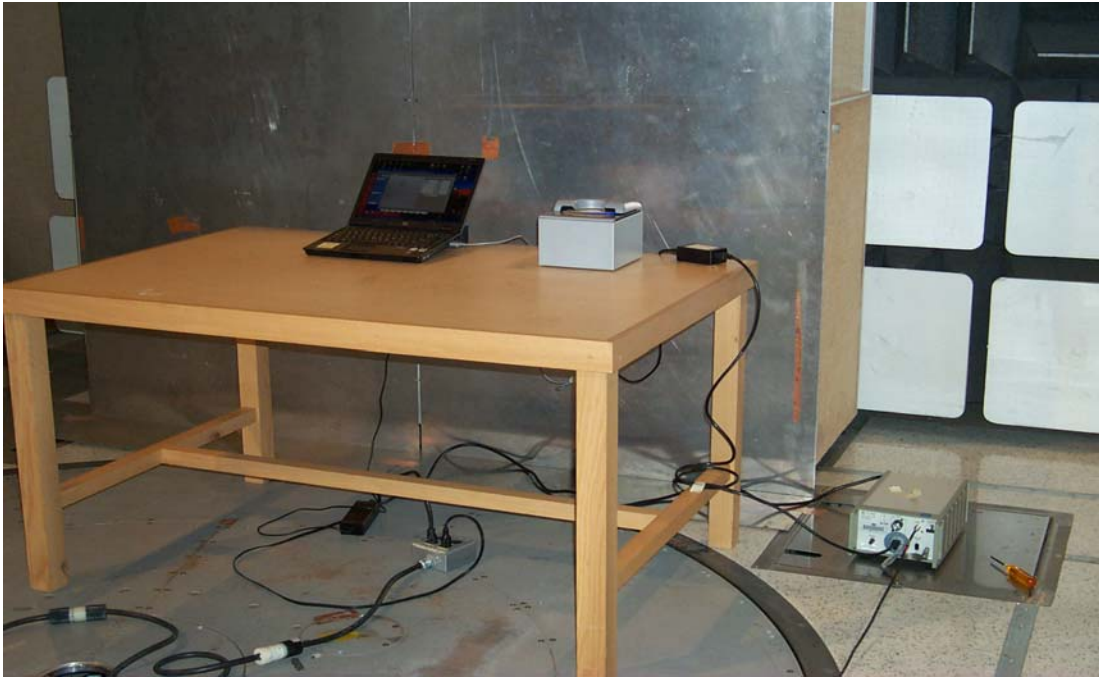
Conducted Emissions Test Setup (RTE8000)
